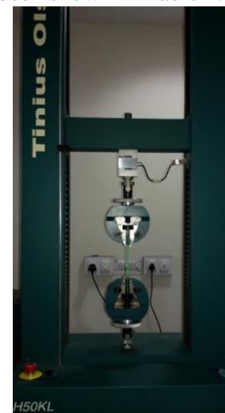
Fig. 2 Experimental setup for tensile testing
