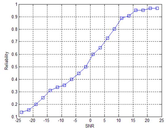
Fig. 2. Reliability of Sensing node with SNR
