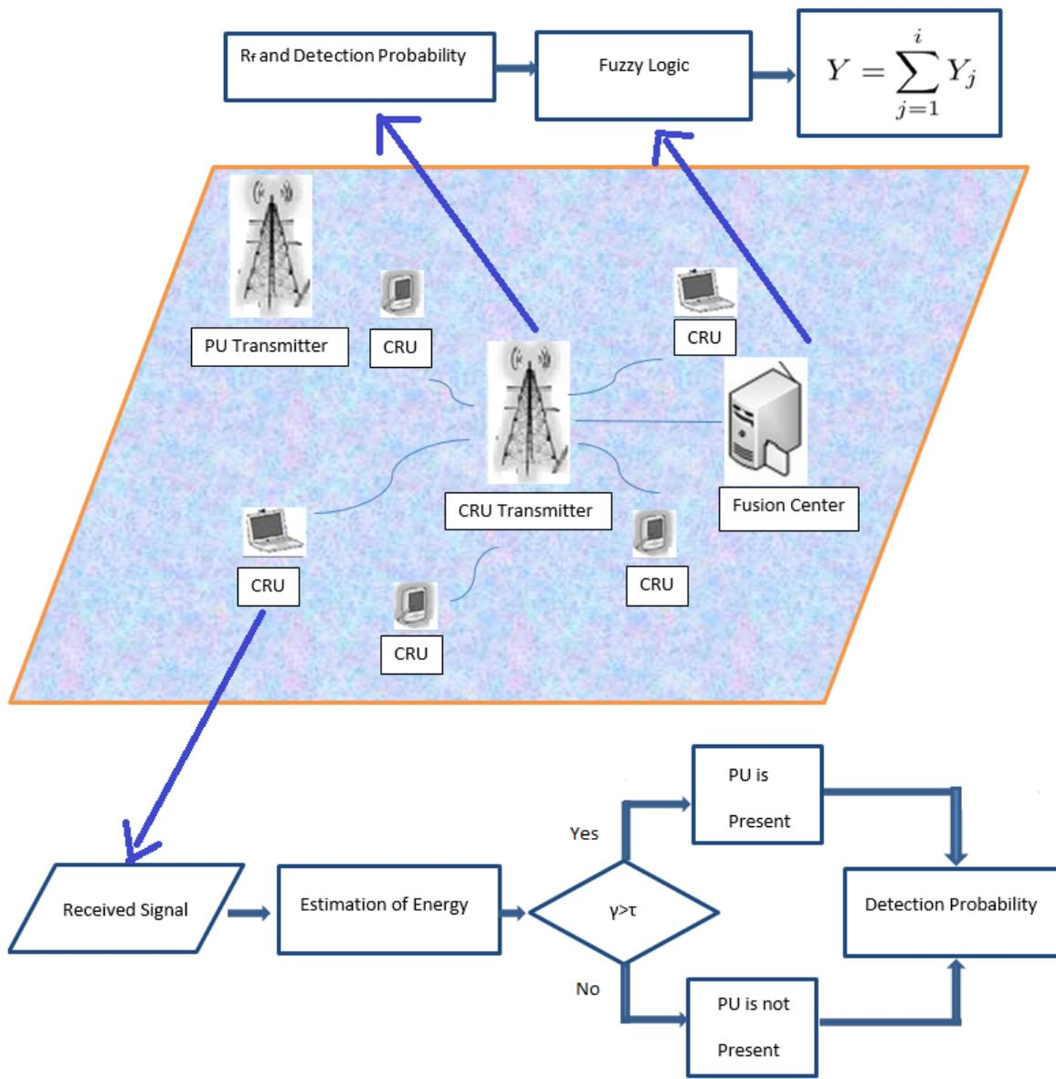
Fig. 1. Proposed RFL Scheme for Spectrum Sensing
