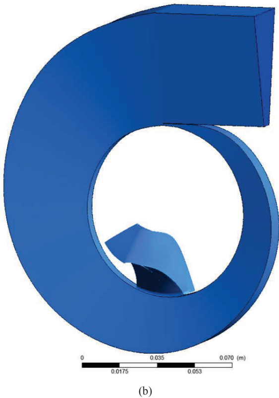
Fig. 6 Volute with one rotor blade: (a) near the tongue and (b) far from the tongue
