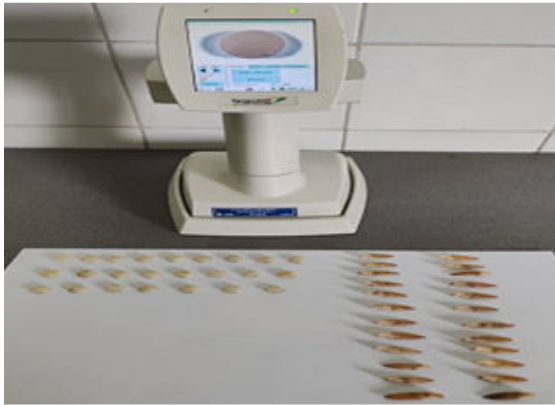
Figure 2: Colorimetric by a spectrophotometer
