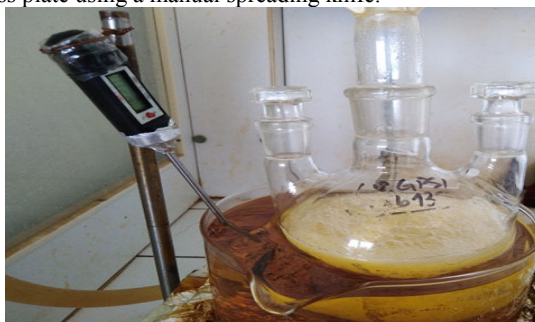
Fig.1. Preparation of membrane at 130°C for 5 hours
