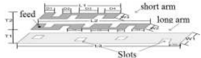
Fig. 2. Geometry of the feed antenna
