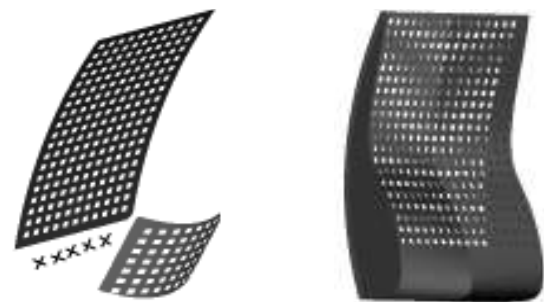
(a) Multi-feeds for multi-beams (b) Covered with a gridded radome
